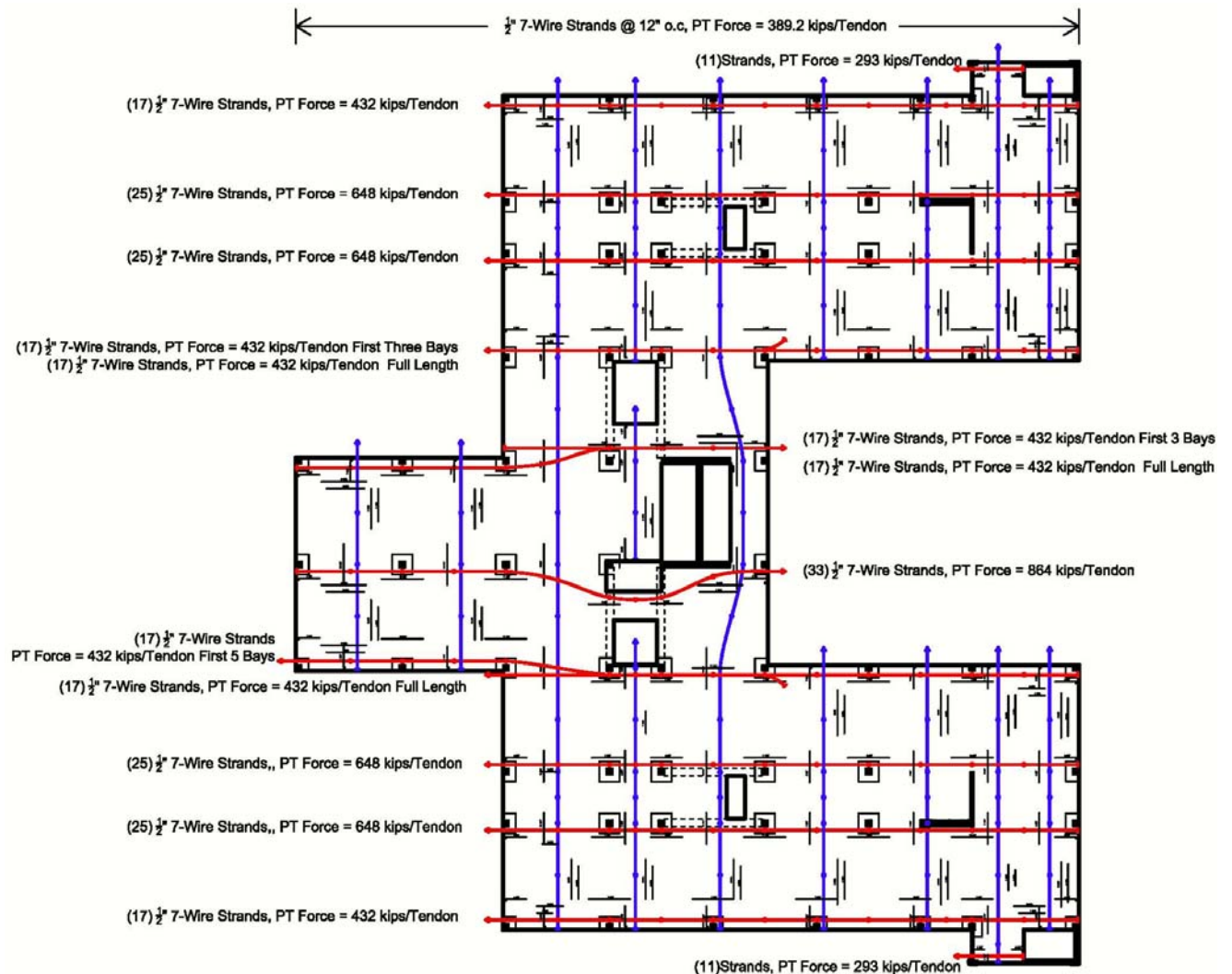
Figure 28: Typical Post-Tensioned Tendon Layout for Shear Wall System
